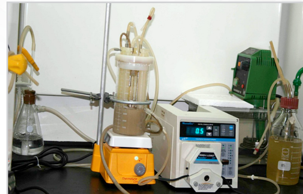
Fig 1: CDC Biofilm Reactor
